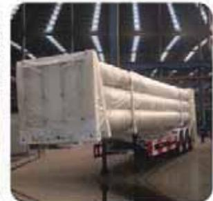
Jumbo cylinder produced as per ISO11120, DOT, or ASME standard, with TPED approval. Jumbo tube container with ADR, IMDG and RID certificate, and inspection report issued by BV, LRS, TUV or equivalent international third-party.
