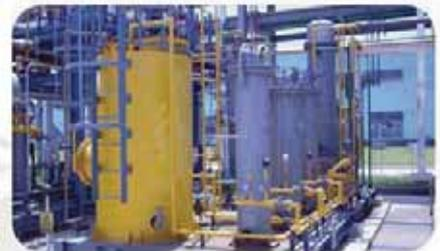
Dehydration and mercury removal Unit
