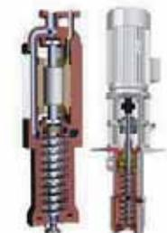
Submerged pump, seal pump
