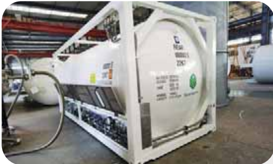
Operation box with pump
